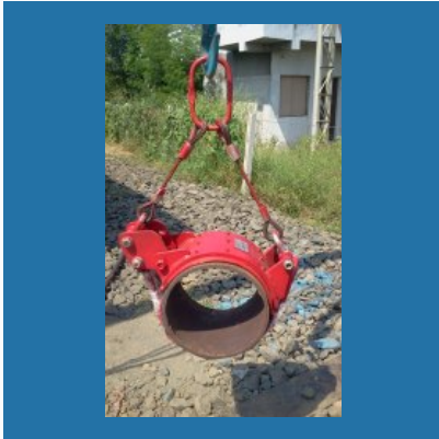
Pipe Lifting Steel Lined Choker Belt
